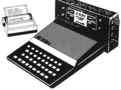
The ZX99 contains its own 2K ROM which acts as an extension to the firmware already resident in your ZX81'S own ROM. The ZX99's ROM contains the tape operating system, whose functions are accessed via Basic USR function calls. Each function has an entry address which must be quoted after the USR keyword. All of the functions can be used in program statements, or in immediate commands (i.e. both statements with line numbers and commands without them).
